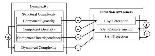
Fig. 3. Model of interface complexity and the mechanisms by which it degrades situation awareness.
