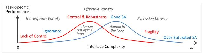
Fig. 1. Optimum interface complexity lies at the intersection of system and human performance functions (i.e. between the red and blue peaks).
